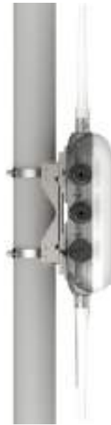
FAP-432G Pole/Wall Mounting
